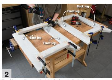
The side top rails are set back 7/8 in. from the front edge of the front legs. The side bottom rails are set back 3-1/4 in. from the front edge of the front legs. Both rails are 2-3/8 in. from the back edge of the back legs.
