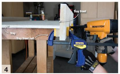
Attach the tray front to the tray front rail with glue and finish nails. Then attach the handles with 1-5/8-in. screws.
